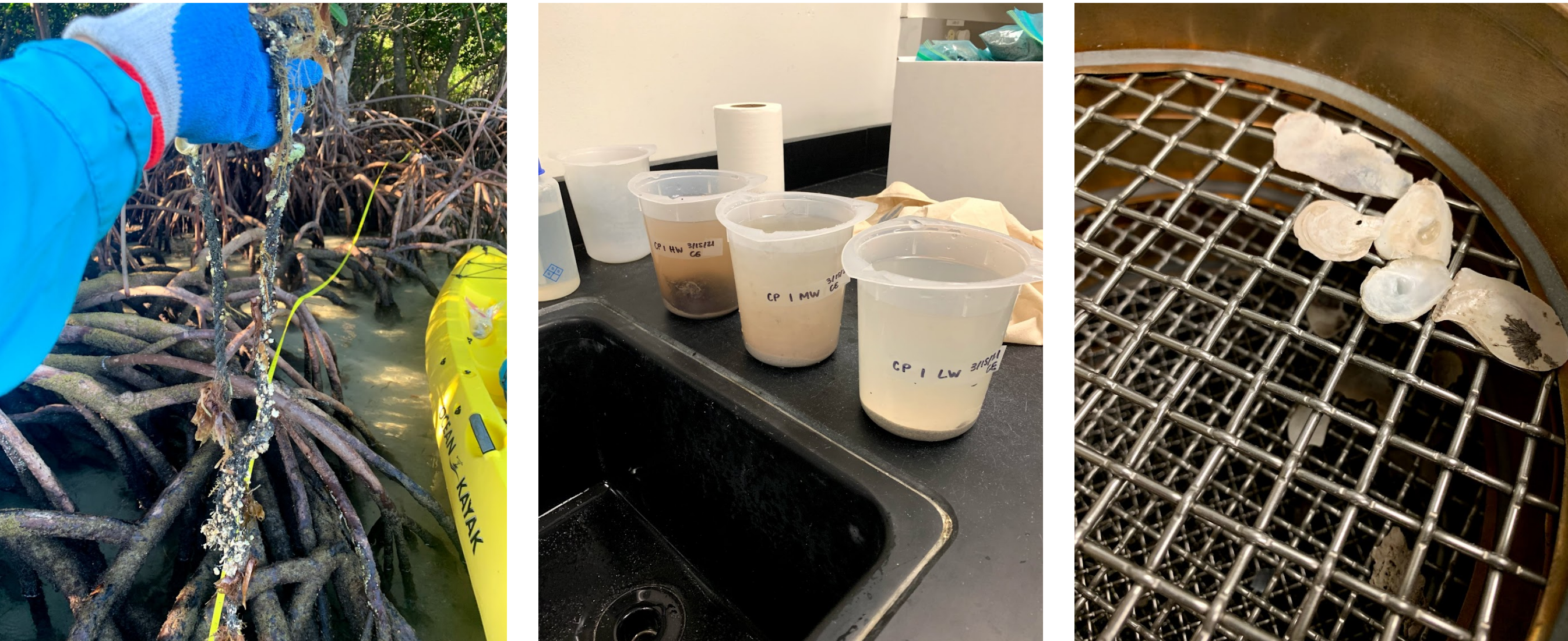
Figure 2 L to R: Fishing gear found along line transect in mangroves, sediment samples being washed to prep for analysis, oyster shells sorted by Ro-Tap.
