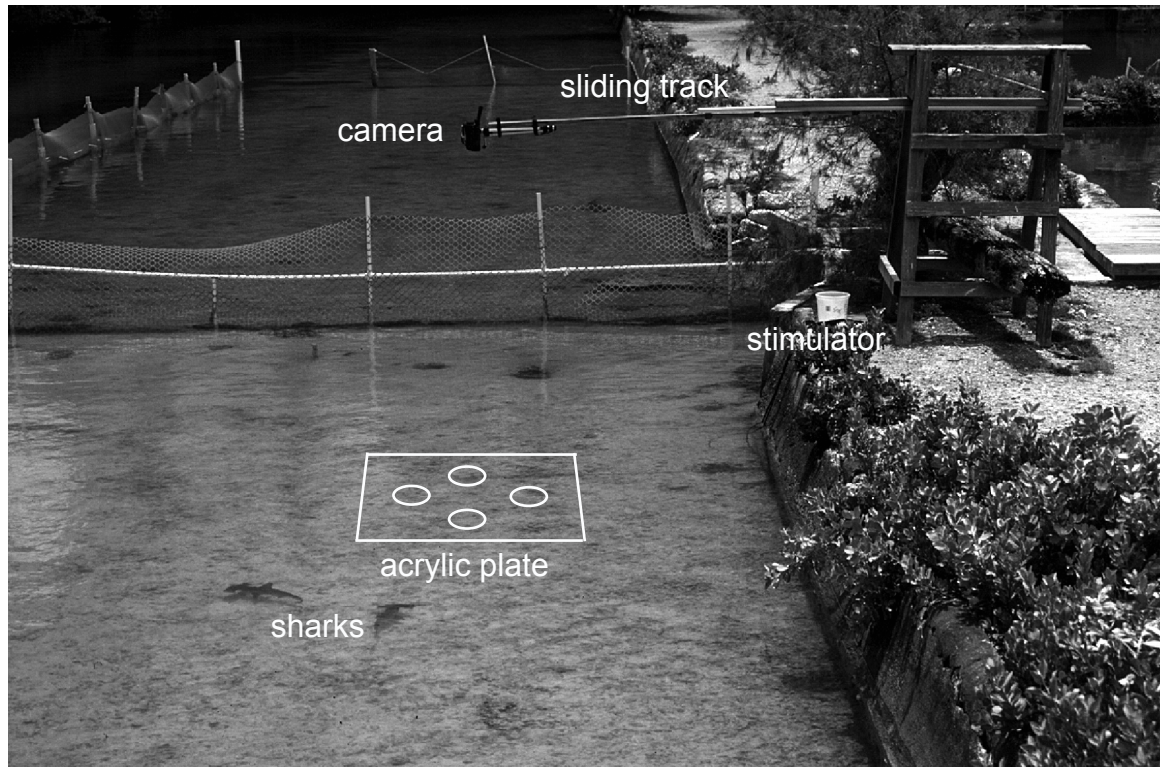
Figure 3.3 Experimental apparatus used to study the response of scalloped hammer-head sharks to prey-simulating dipole electric fields. One of the four electrode pairs (circles on the acrylic plate) was activated with a weak electric current which generated a dipole electric field around the electrodes. The response of the sharks was videotaped with a camera affixed to the end of a sliding track and positioned directly above the center of the electrode array.
