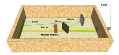
Teams will be provided three mirrors and an eye safe Class 3b red laser. The light must strike each of the three mirrors before hitting the target and there may be obstacles that the beam of light will have to be directed around. (see sample diagram)
