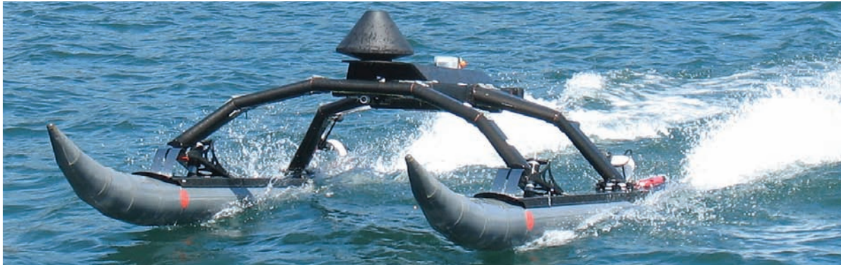
Autonomous unmanned surface vehicles, like the WAM-V catamaran, are being developed with funding from the Office of Naval Research.
