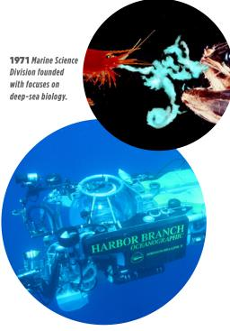
1971 Built in 1971 and 1975, the Johnson Sea-Link Submersibles revolutionized the field of deep-sea exploration with their large, acrylic spheres which allowed a near-360-degree view of life under the sea. These submersibles were in commission for nearly 40 years, and together conducted more than 9,000 dives worldwide. led by more than 3.000 scientists.
