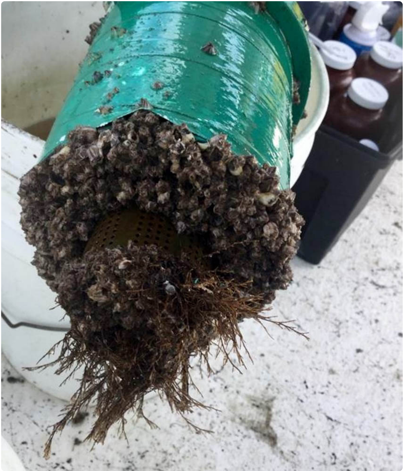
Three weeks of heavy barnacle and bryozoan growth on the sensor end of SeaFET, which measures pH, resulted from lowered salinities following an unusual rain event at our "Crossroads" site (IRL-SLE), October 12, 2015. (Image credit: Kristen Davis)
