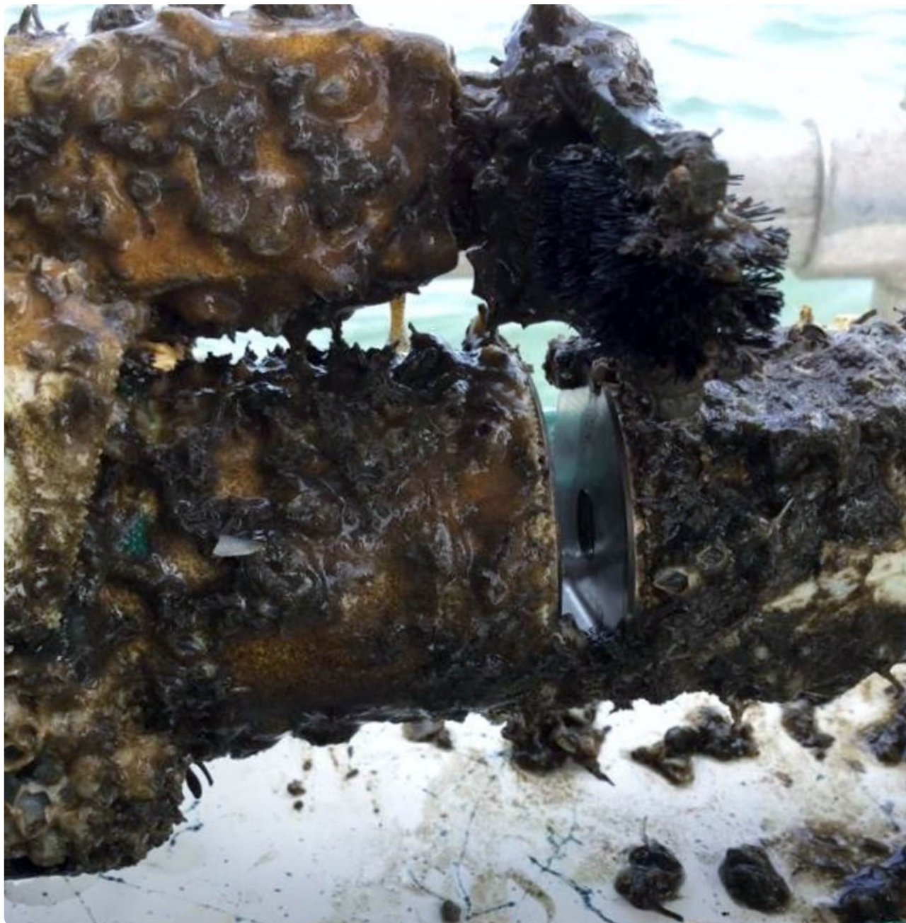
Heavy growth and sedimentation are evident on this SUNA, which measures nitrate, and its integrated wiper, after three weeks at our Link Port site (IRL-LP), near Harbor Branch, July 25, 2015. (Image credit: Kristen Davis)
