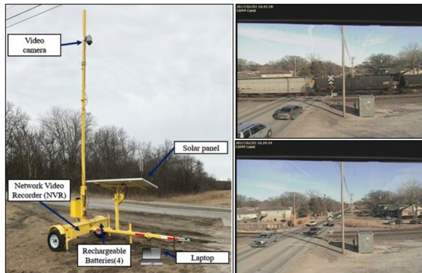
Figure 4.2 Configuration of data collection equipment for train activity data (left) and field-of-views from the installed IP camera (right above and below)
