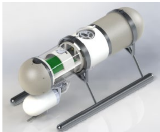
Figure 3. Bio-Inspired Autonomous Underwater Vehicle to Detect, Track and Follow a Surface Moving Object.
