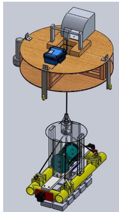
Figure 2. Remote Concrete Mattress Deployment Frame.
