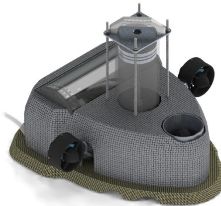
Figure 4. Bio-Inspired Self-Burying Autonomous Underwater Vehicle.
