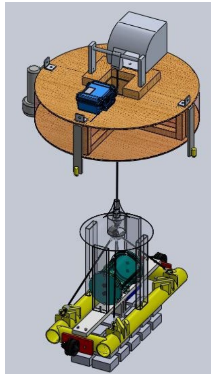
Figure 2. Remote Concrete Mattress Deployment Frame.
