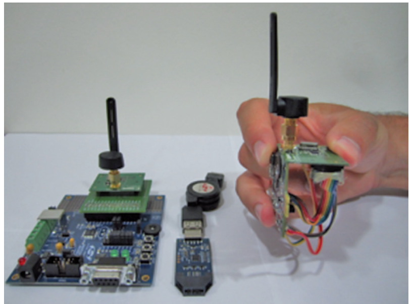
Figure 2. The portable transceiver iCube v0.1, developed for the course (on the right). It consists of a low-cost radio module interfaced to an MCU unit small-form-factor development kit. On the left are the AA-battery holder, the MCU toolstick USB programmer, and a radio module interfaced on an MCU development kit.
