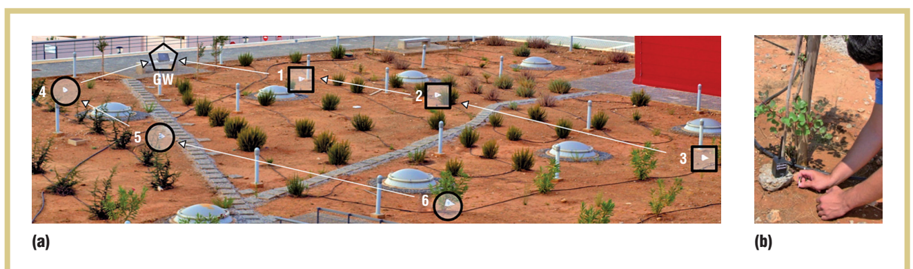
Figure 7. The wireless network deployed outdoors for demonstration purposes. It has (a) two chains (chain 1 in rectangles and chain 2 in circles) and seven nodes and (b) a soil wetness sensor. No special iCube mounting was performed.
