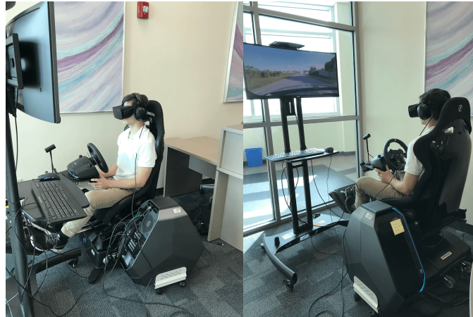
Figure 1: Participant using the SDC simulator.
