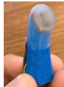
Figure 2 . Fabricated TakkTip sensor for measuring the forces of all experiments in this paper.
