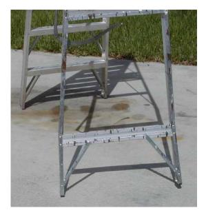
Figure 6: Type II Racking failure.
