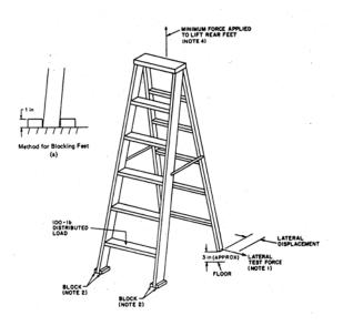
Figure 3: Racking Test according to [1]
