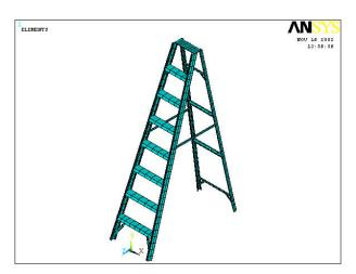
Figure 2: Ladder's finite element model.
