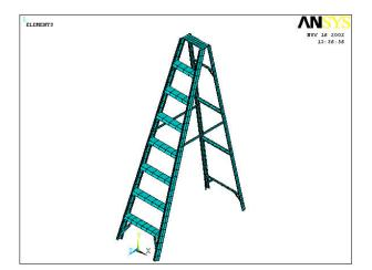
Figure 2: Ladder's finite element model.
