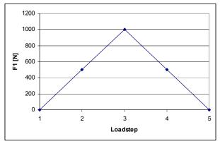
Figure 8: Discretization of the impact load.
