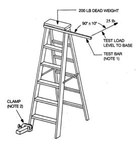
Figure 4: Torsion Stability Test.
