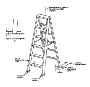
Figure 3: Racking Test according to [1]
