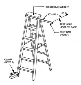
Figure 4: Torsion Stability Test.
