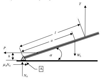
Figure 4: Free body diagram of a suspended ladder.
