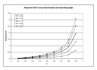
Figure 3: Required COF at point A to avoid slippage.
