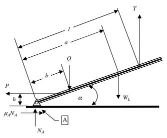
Figure 5: Additional load to the system of Figure 4.
