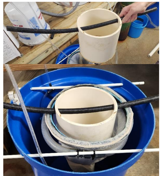
Figure 49. Detail of prefilter (inset at top) and its placement in the filter sock of the harvest tank.
