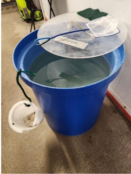
Figure 47. Disinfection Barrel with 10% sodium hypochlorite solution. Note the surplus pump basket for small part disinfection hanging on the outside of the bucket for the parts to dry.
