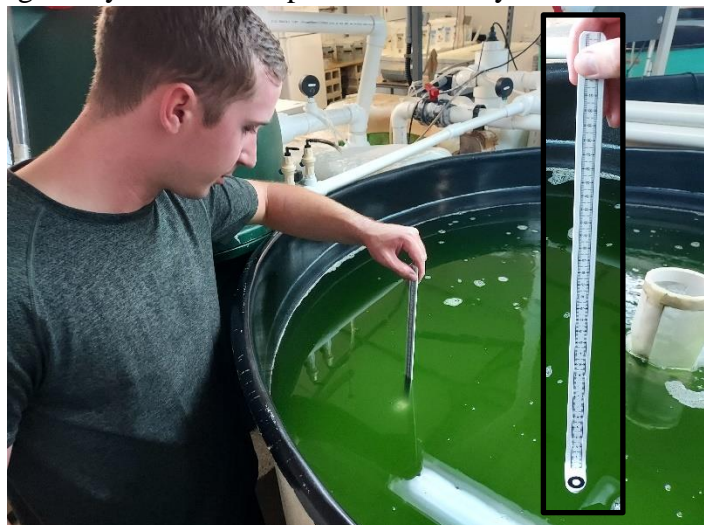
Figure 57. Handheld Secchi disc device used to measure turbidity due to the greening compound (detail of device inset).
