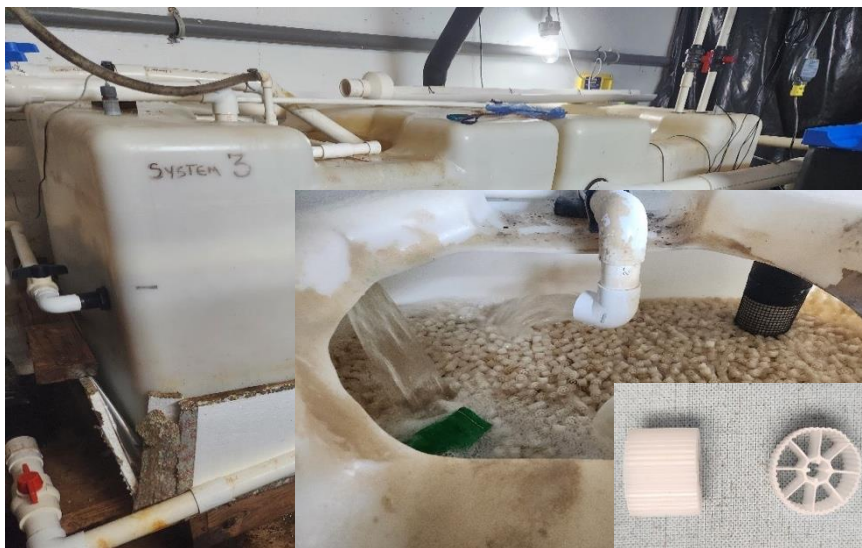
Figure 20. Dual sump/moving bed biofilter with MB3™ bio-media in one tank.
