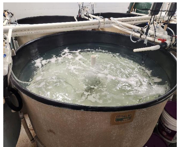
Figure 43. Closeup view of larval rearing tank. Note: light colored bottom and black sides.
