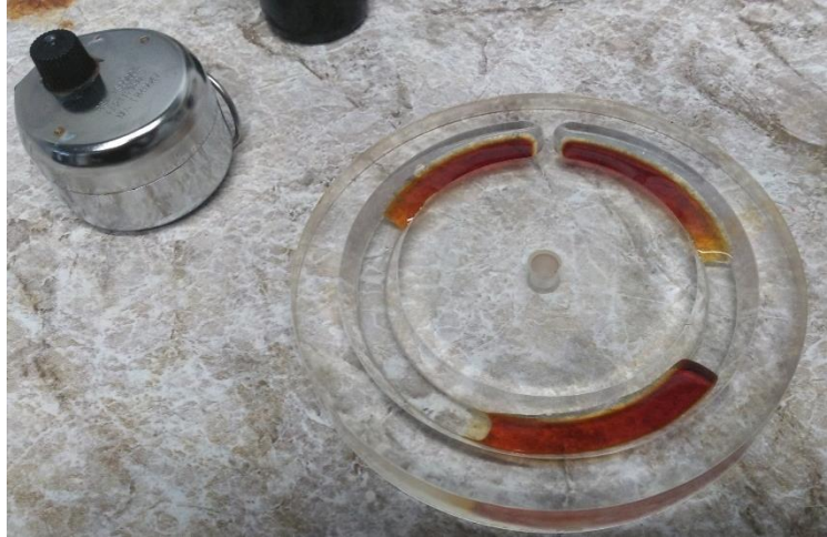
Figure 45. Ward Counting Wheel with three 1 ml samples of rotifers stained with lugol's solution.
