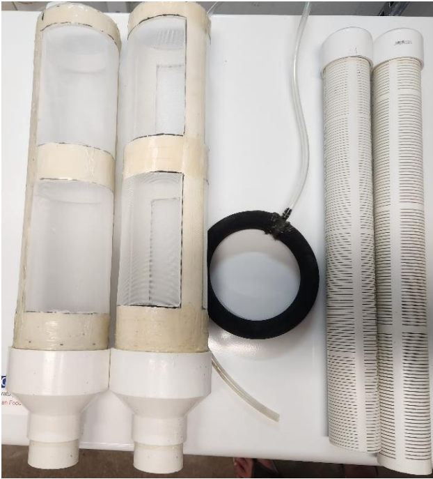
Figure 44. Screens (left to right 250 µm and 500 µm), bubble curtain, and slotted pipes (from left to right 800 µm and 1,200 µm) used during the larviculture period for pompano from egg through weaning.
