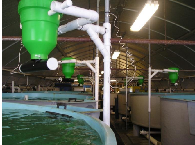
Figure 60. Automatic feeders on experimental production tanks at HBOI-FAU, Fort Pierce FL.
