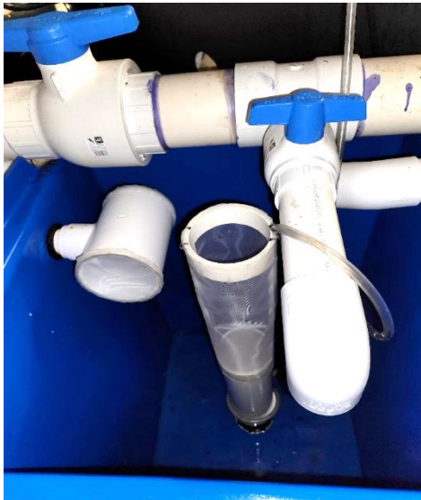
Figure 34. View of egg collector showing nylon screen filter elements and bubble screen in place ready for a spawn once flow is diverted.
