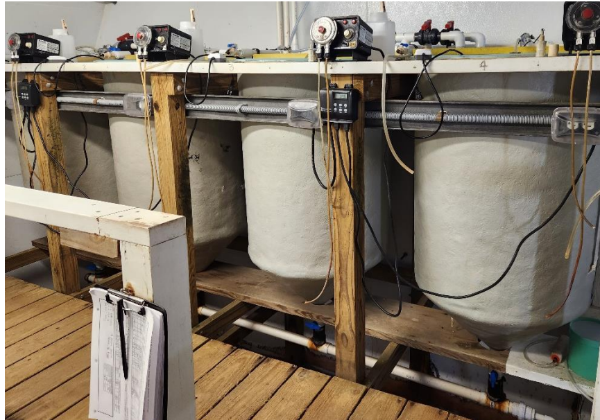
Figure 50. 400 L Rotifer tanks on stand. Note: Harvest drain line manifold at bottom with individual valves for each tank (blue)
