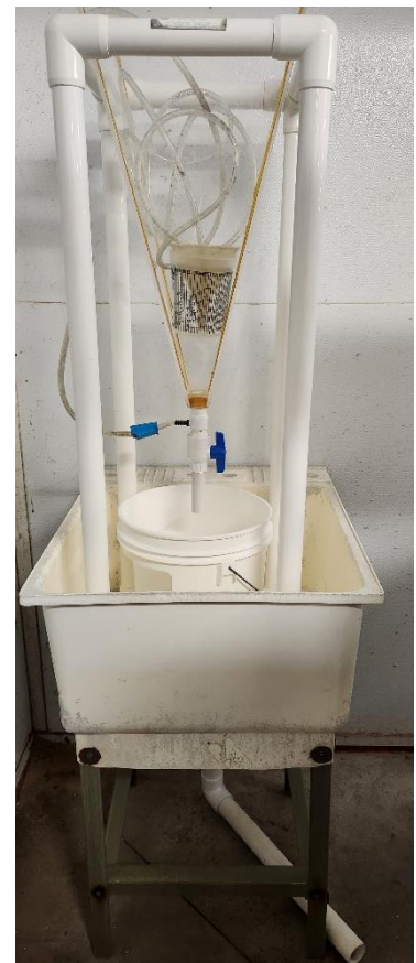
Figure 55. Artemia decapsulation cone with stand setup in a sink dedicated to the process.
