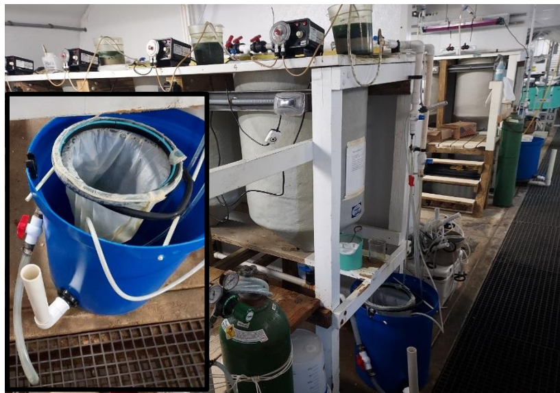
Figure 48. Detail of Rotifer harvest tank (inset on lower left) and placement at end of culture tank drain manifold. Prefilter sieve is shown on the stand to the left of the harvest tank in the main picture. Note: Main drain manifold valve is the red handled valve to the left of the rotifer harvest tank It is shown resting outside of the harvest tank in these photos.
