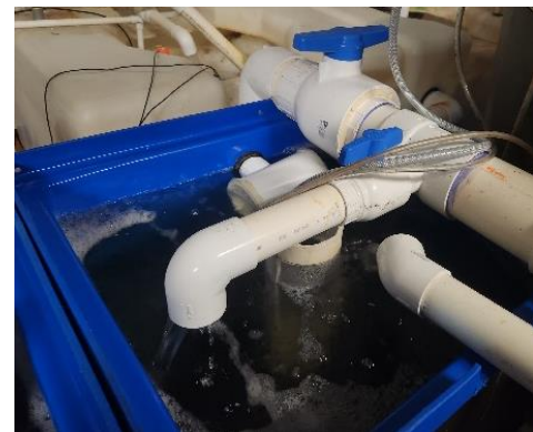
Figure 35. Egg collector box with flow diverted from tank in preparation for egg collection.
