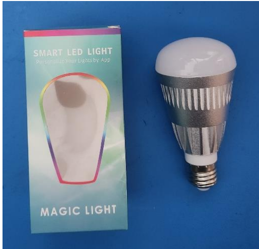
Figure 21. Example of one brand of Smart LED light that uses a standard Edison screw type socket.
