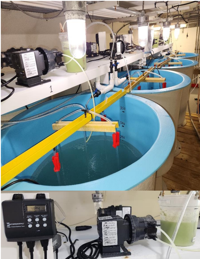
Figure 46. Rotifer culture tanks. Note detail inset at bottom of Peristaltic pump for metering feed to the rotifers from the feed container.
