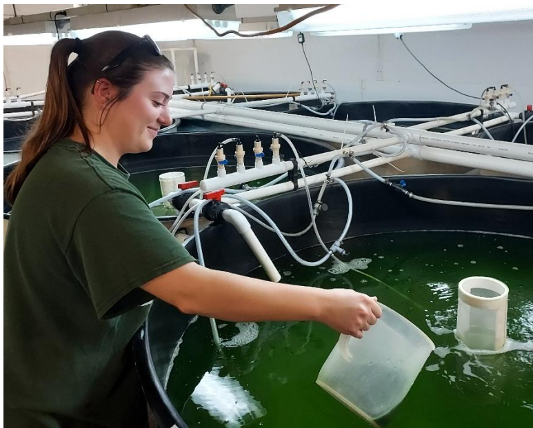
Figure 58. Adding greening agent to the larval tanks.
