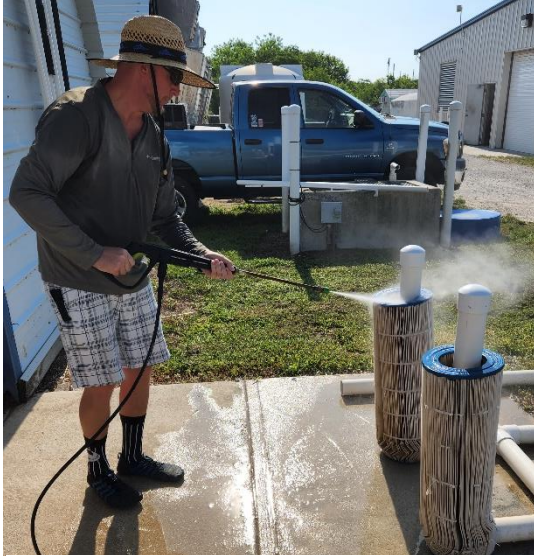
Figure 25. PVC stand constructed to facilitate pressure washing of pleated paper filter cartridges for reuse.
