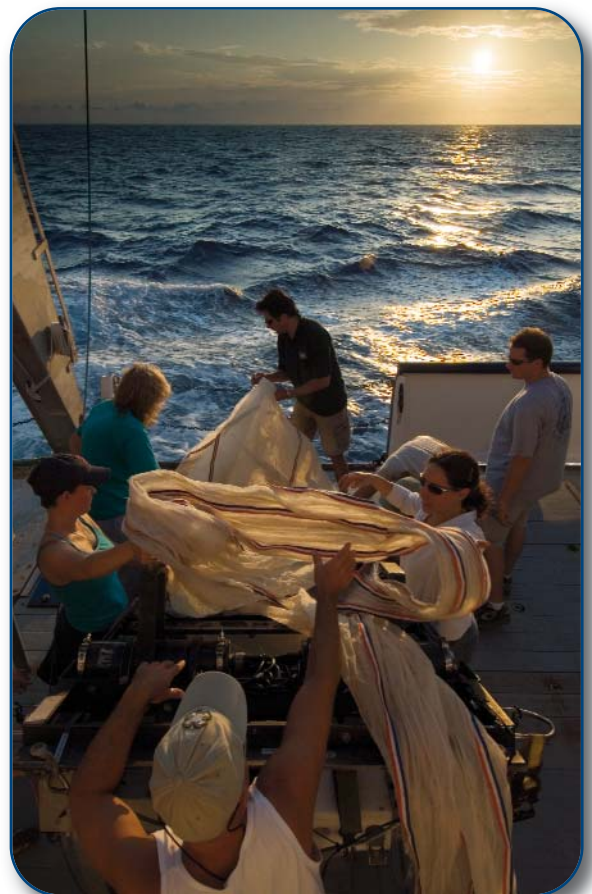
The MOCNESS Trawl – a large net used to gather deep water organisms and bring them to the surface unharmed is an example of the technology developed by Harbor Branch.
