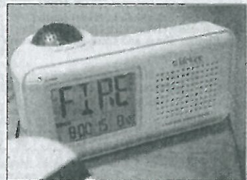
GARY CORONADO / THE PALM BEACH POST One local deaf couple was given an alarm that flashes 'FIRE' and activates an intermittent bed shaker that is placed under the mattress.
